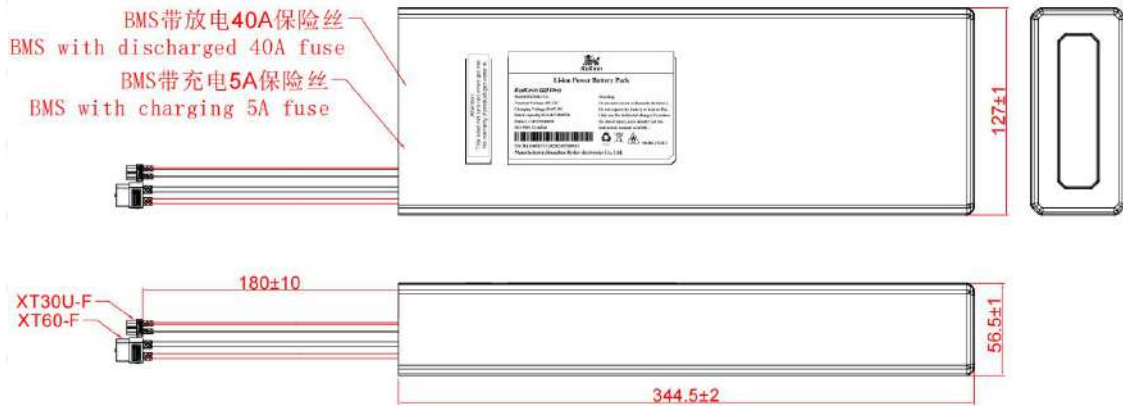
Battery (Unit: mm)
